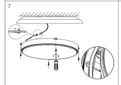
Connect the base and led module. Align the screw holes of base and led module, fix the led module on the base firmly by screws.
