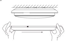
Match the gaps for each part and rotate the frame clockwise.
