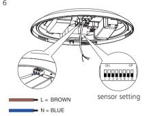
Connect the wires to the block through the reliefs.
