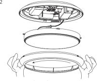
Unscrew the front frame anticlockwise and take it out, make the frame, diffuser and back housing separately.
