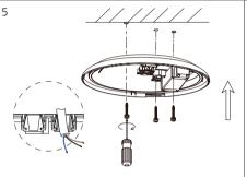
Make the input wires through entrance hole and waterproof bushing, cover the screws with waterproof washer, fix the back housing by these screws.
