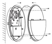
Connect the DC plug( if with Emergency , connect the plugs between the battery and driver), put back the cover to the back plate and fix it by screws  $\frac{1}{2} \int_{-\infty}^{\infty} \frac{1}{2} \left( \frac{1}{2} \int_{-\infty}^{\infty} \frac{1}{2} \left( \frac{1}$
