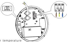
Choose the color temperature with DIP switch if it's the color changeable version, then connect the wires well.
