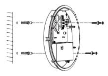
Fix the back housing on the wall or ceiling by screws.
